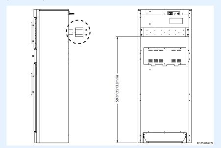
If floor mounting, **bolt** the warmer to the floor using facility approved fasteners (not included) or contact Customer Service for optional floor mounting hardware.
