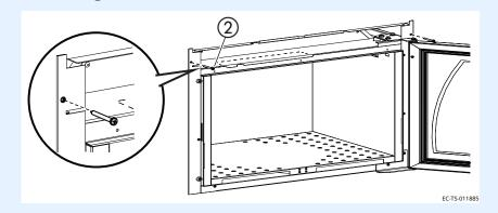
5. **Re-install** the interface assembly. **Make sure** all of the tabs lock the interface bends into place.
